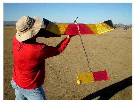
In position for an overhand launch using the two handed techique. Keep the model pointed UP and give it a firm but controlled push. It's best to have the wing tilted down slightly toward the turn direction you want the model to transition into.
