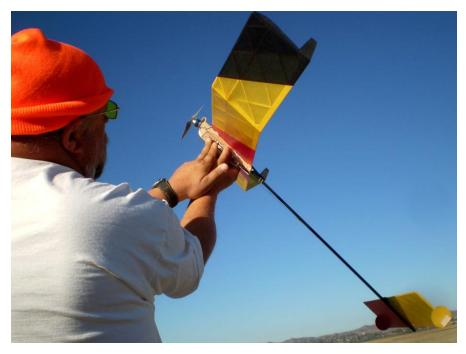
Stan Buddenbohm holding the model with the two handed grip that feels right for him. Note the difference between my direct index finger contact on the start button and his that encompasses the launch hand as part of his way of stabilizing the launch attitude of the model.
