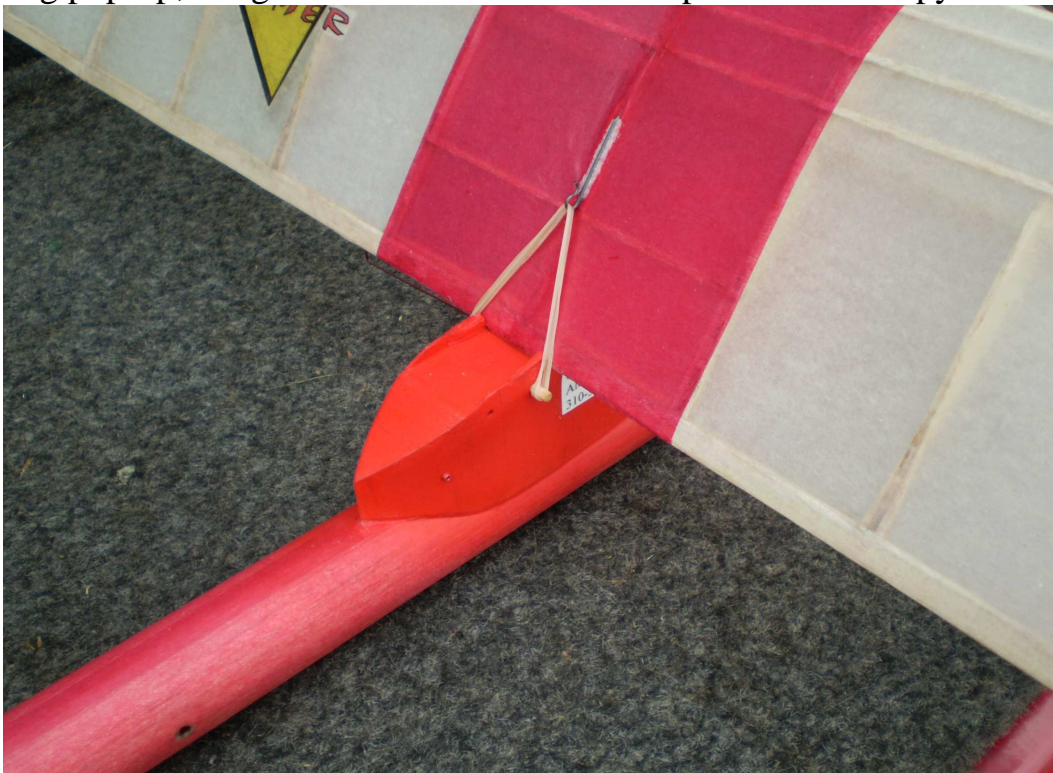
Wing pop-up right side detail; note T.E. stops and notching
