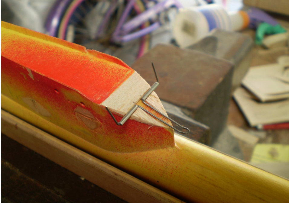
Trip wire assembly installed
