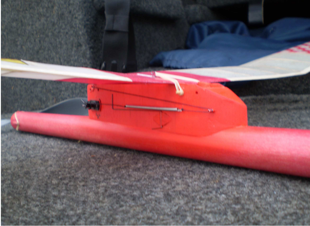
Wing D/T armed-stab tripwire ready to load
