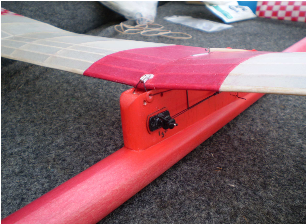
Another view of the wing D/T armed and ready to fly-I countersink the fairlead holes a bit to ease the wear on the lanyard.
