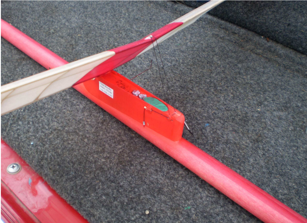
Wing pop-up; bung tube installation-note L.E. pencil mark on pylon floor
