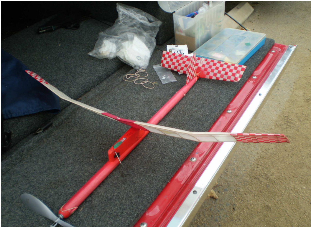
D/T configuration in flight-wing will remain parallel with ground
