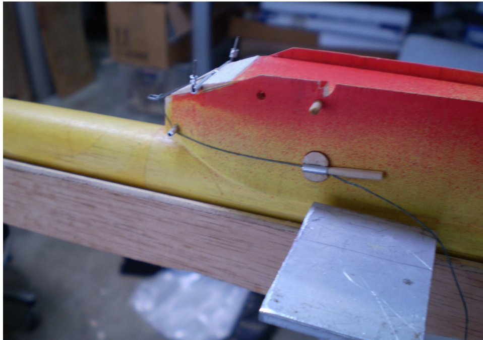
Armed system-bung tube and plug (temp plug shown)
