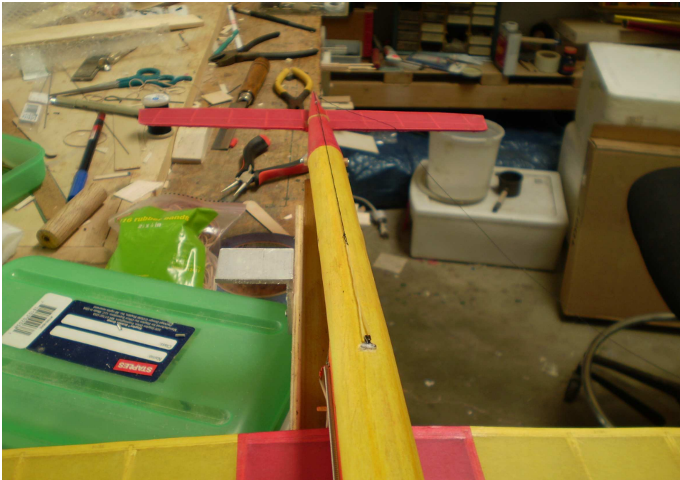
Stab pop-up lanyard secured for retrofit
