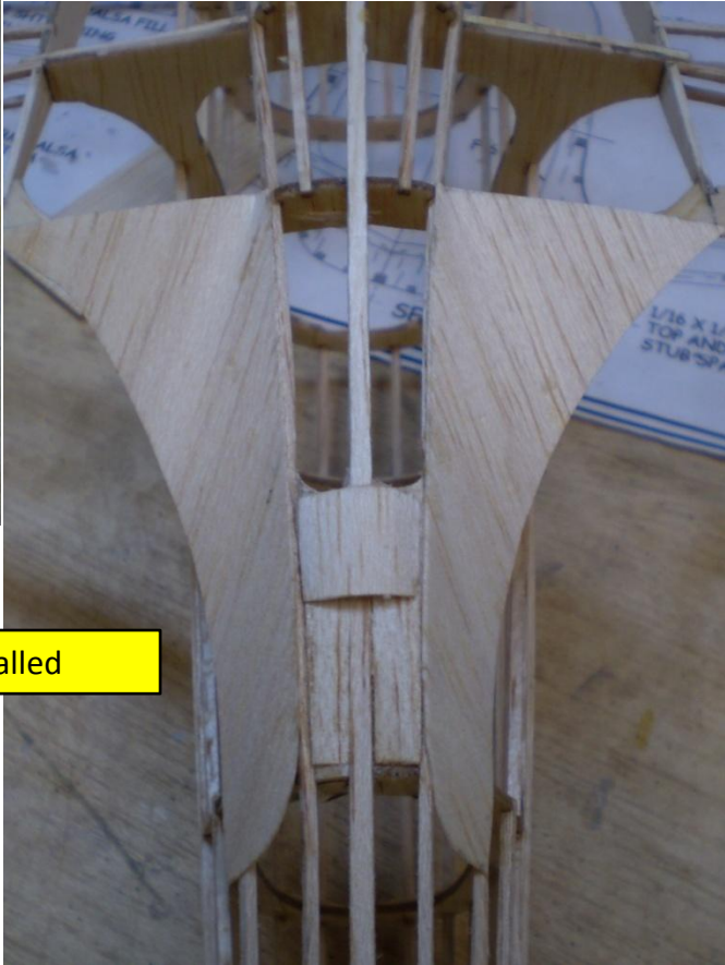
View from the top of the fuselage-inside of lower fillet skin attached to stringer and WF-1
