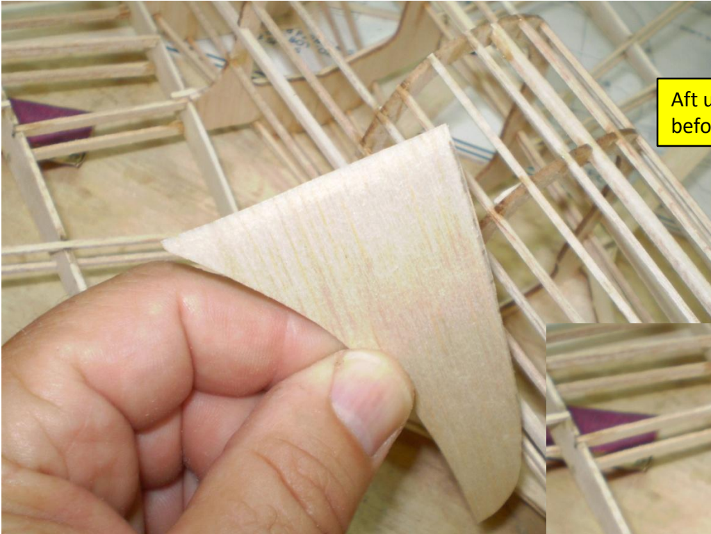
Scarf area is constant width to a knife edge-about 1/8" wide
