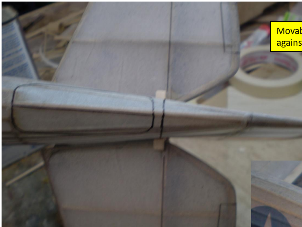
The upper movable shim installed. Position the upper and lower shims until the stab is centralized in the slot and are fairly snug. Don't cram them in or you will deflect the structure and break something-very light pressure to hold them in place. These eventually get bonded lightly in place and trimmed off once you are satisfied with the glide and power trim you have achieved.
