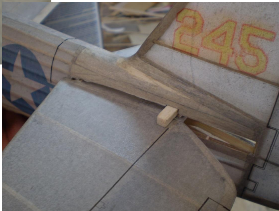
The upper movable shim installed. Position the upper and lower shims until the stab is centralized in the slot and are fairly snug. Don't cram them in or you will deflect the structure and break something-very light pressure to hold them in place. These eventually get bonded lightly in place and trimmed off once you are satisfied with the glide and power trim you have achieved.
